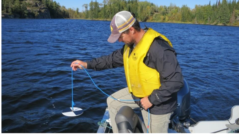
Figure 2 – Lowering of Secchi disk
